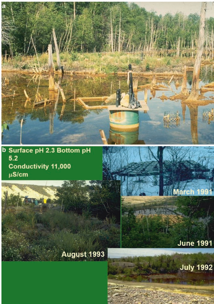
Fig. 6.2 (a) Slow-flowing acid drainage forms a shallow pool at the foot of a tailings dam in Elliot Lake. The site was selected to test if secondary minerals could be detected in constructed sediments placed into highly acid water. The drums contained organics and rusty nails with straw. Porewater was sampled under nitrogen gas to examine if authogenic minerals could be found under the microscope, nettings without rusty nails formed as a control. (b) The alfalfa bails were placed in a honeycomb structure to allow reducing and oxidizing heterotrophic microbes to invade the bails. In March 1991 the bails were placed on the ice as access was otherwise not possible. In July 1992 the structures had remained but by August 1993 vegetation had invaded and the bottom pH had improved from 2.3 previous to 5.2. Note the high conductivity which had not changed. (Photographs by Boojum Research)
